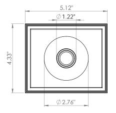
Ceiling Cut-Out: 4.49" x 5.28" Fixture Dimensions
