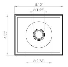
Ceiling Cut-Out: 4.49" x 5.28" Fixture Dimensions
