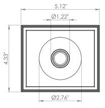
Ceiling Cut-Out: 4.49" x 5.28" Fixture Dimensions
