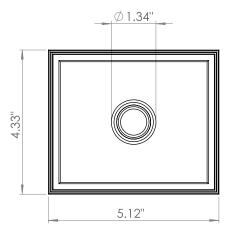
Ceiling Cut-Out: 4.49" x 5.28" Fixture Dimensions
