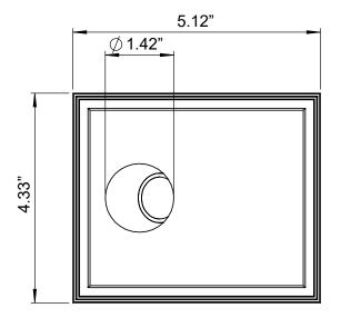
Ceiling Cut-Out: 4.49" x 5.28" Fixture Dimensions
