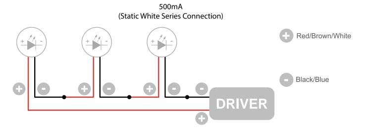
The individual lamps must be connected in series. Only power up the system once all the lamps have been connected.
