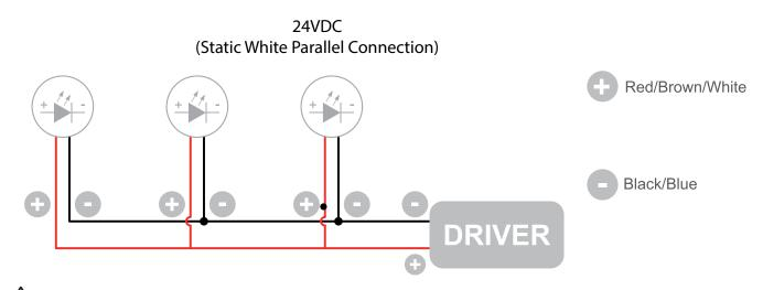
The individual lamps must be connected in parallel. Only power up the system once all the lamps have being connected.
