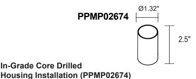
Drill pilot hole for core drilled housing through concrete and into soil below Create appropriate pathways through soil for running wires from fixtures to drivers
