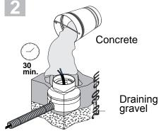
Use 7-12" of drainage gravel - check functionality: fill tube with water and verify full drainage within 30 min. If water remains, please utilize a different drainage system that functions properly. Contractor to seal the conduit with "Great Stuff" aerosol seal that prevents water and moisture penetration for ultimate protection.
