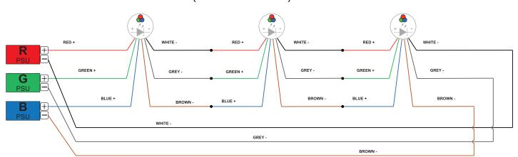
FOR RGB VERSION ONLY: The individual lamps must be connected in series. CURRENT Only power up the system once all the lamps have being connected.
