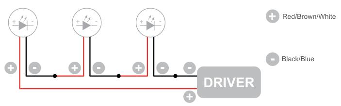
The individual lamps must be connected in series. Only power up the system once all the lamps have been connected.
