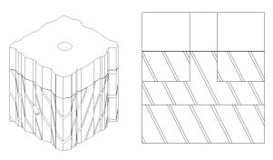
Apply epoxy to sides of newly drilled opening, insert core drilled housing into pilot hole and make level
