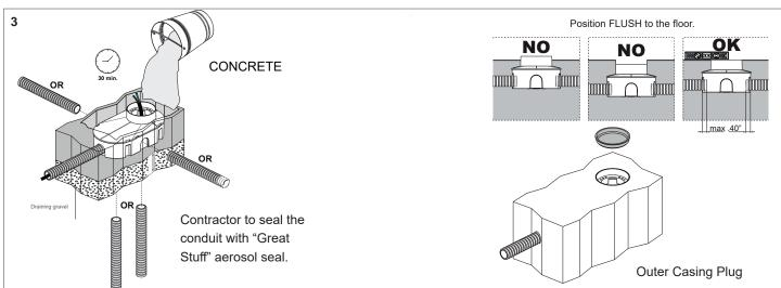
Use 8" of drainage gravel - check functionality: fill tube with water and verify full drainage within 30 min. If water remains, please utilize a different drainage system that functions properly.
