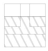
Apply epoxy to sides of newly drilled opening, insert core drilled housing into pilot hole and make it level
