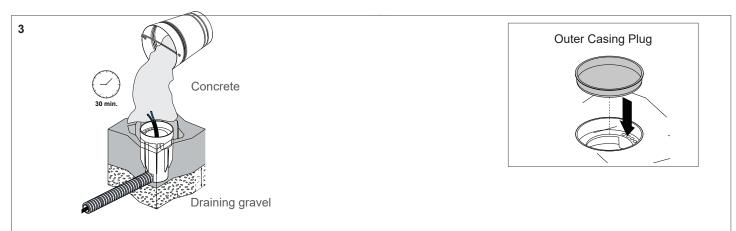
Use 8" of drainage gravel - check functionality: fill tube with water and verify full drainage within 30 min. If water remains, please utilize a different drainage system that functions properly. Contractor to seal the conduit with "Great Stuff" aerosol seal that prevents water and moisture penetration for ultimate protection.
