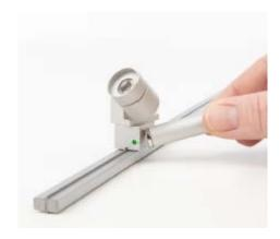
Place the dimmer pin in the sensor area. As soon as the green feedback LED at the cable input lights up, the sensor is activated and the spotlight is dimmed. The dimming process stops when the pin is removed. The dimming direction is changed when the dimmer pin is applied again.
