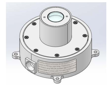
\* Housing is tapped on the sides with two (2) NPT threads for conduit or IP68 liquid tight fittings. Properly plug and seal the threads using **TEFLON plumbers tape or equivalent thread sealer** to prevent water from entering the housing. *A conduit plug is supplied but not sealed!!!*
