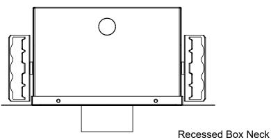
It is contractor's responsibility to arrange power wires into box before concrete is poured.
