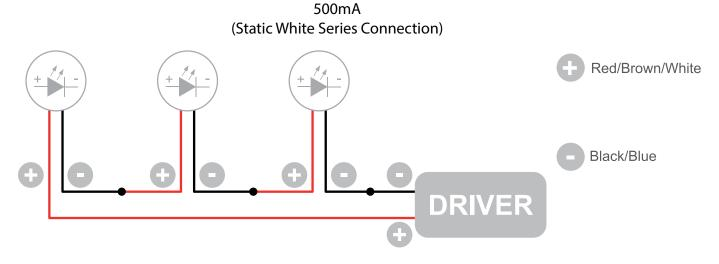
The individual lamps must be connected in series. Only power up the system once all the lamps have been connected.
