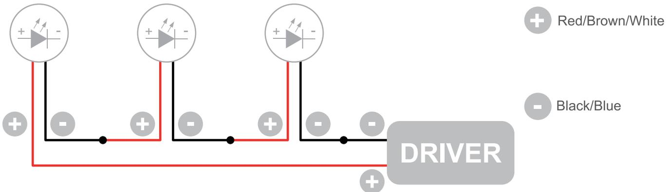
The individual lamps must be connected in series.
