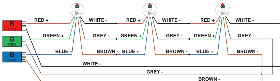
The individual lamps must be connected in series. Only power up the system once all the lamps have being connected.
