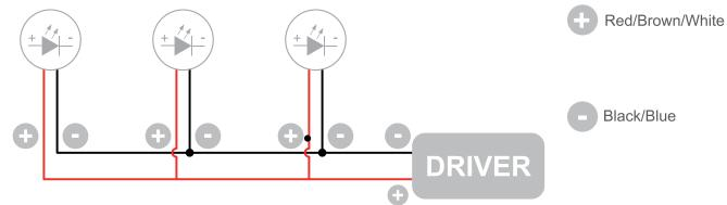
The individual lamps must be connected in parallel. Only power up the system once all the lamps have being connected.
