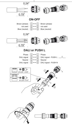
After wiring, tighten cable gland "B" on trim "A", then insert grommet "C" on cable gland "B". Finally, firmly fix nut "D" on cable gland "B".
