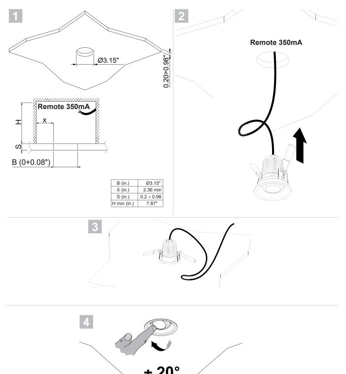
It is the contractor's responsibility to install Remote Driver in a suitable electrical enclosure.
