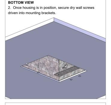
4. Attach the fixture to the face plate as shown. Connect fixture wires to building wires, **RESPECTING POLARITY.** Mount the assembly into the back box. Adjust accordingly so the fixture face is flush with the ceiling surface.
