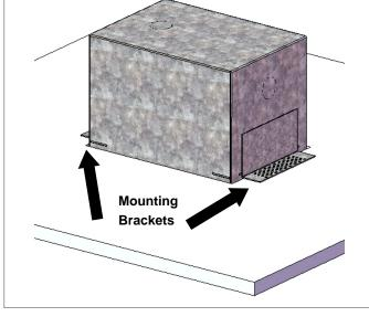
3. Loosen all four wingnuts slightly and position the housing so that is it recessed in the opening by about ¼". Tighten all wingnuts
