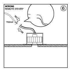
• Use gel-filled waterproof wirenuts for wire connections.
