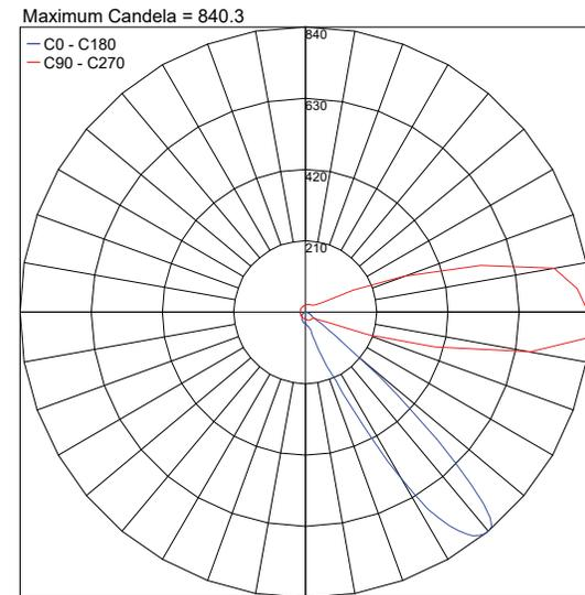
PHOTOMETRIC FILENAME : GENIUS BASIC SLOPE BU1865.00 500MA 3K.IES
