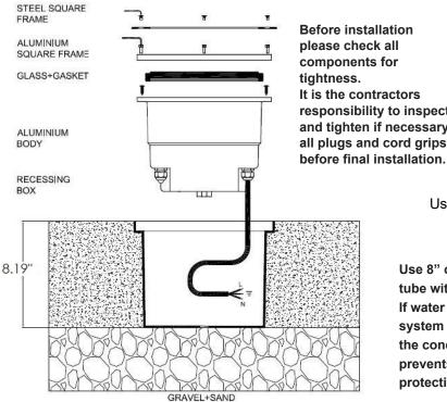
Before installation please check all components for It is the contractors responsibility to inspect and tighten if necessary all plugs and cord grips
