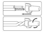
Use gel-filled waterproof wire-nuts for wire connections.
