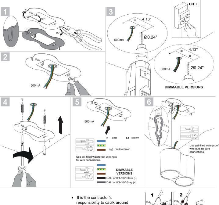
It is the contractor's responsibility to caulk around the edges between the fixture and the mounting surface, to satisfy wet label requirements.
