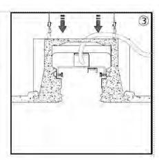
Use gel-filled waterproof wirenuts for wire connections.
