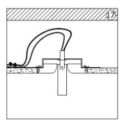
Use gel-filled waterproof wirenuts for wire connections.
