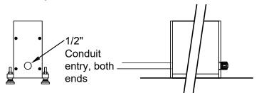
Use optional adjustable leveling pads (LL301) for additional leveling of outer housings.
