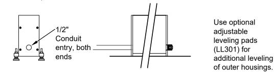
4. Using wire-tie, secure the outer body (i.e. to rebar or the like) in such a way as to ensure that the body cannot move when the concrete is poured.
