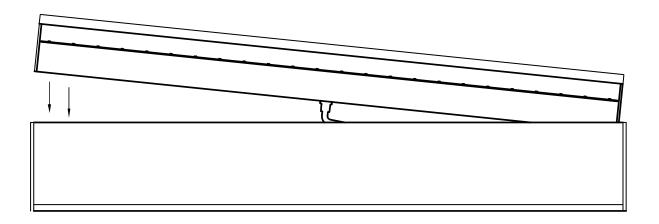
7. Apply a bead of silicone sealant in the hairline gap between the inner and outer body housing. This prevents dirt, grime and other debris from caking into the gap.
