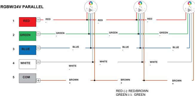
COLORS MAY VARY BASED ON FIXTURE; ALTERNATE WIRING CONFIGURATIONS SHOWN BELOW
