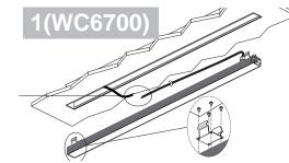
Connect to mains power using a suitable terminal board inside a connection box with the correct ingress protection, in accordance with systems regulations.
