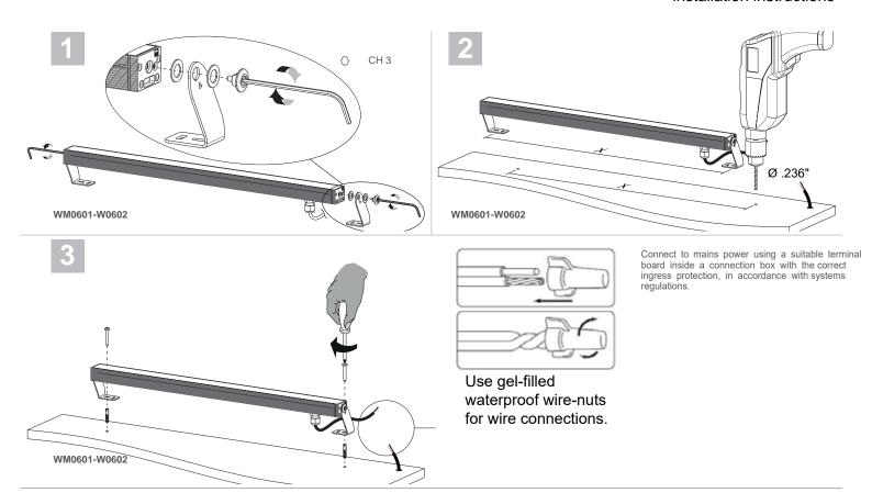
• It is the contractor's responsibility to caulk around the edges in between the fixture and the mounting surface, to satisfy wet label requirements.
