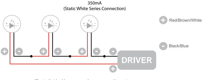
The individual lamps must be connected in series. Only power up the system once all the lamps have been connected.
