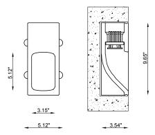
The Passé IP65 is a recessed wet label wall or ceiling mounted fixture made of DurCoral® which is perfect for path or wall lighting. It is unfinished for painting and available in white light with 70° wide beam optic.
