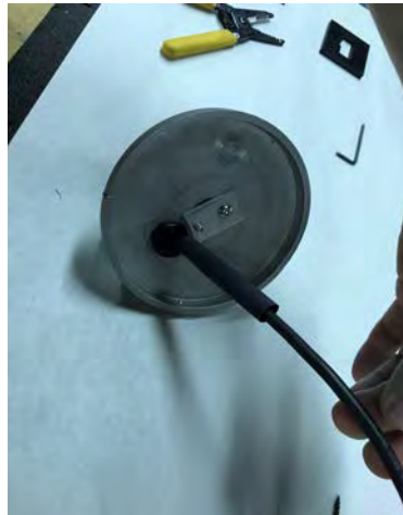
Fixture cord after modification
