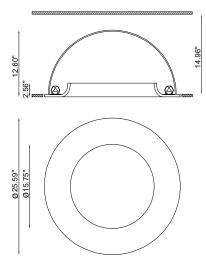
light, rounded edge and a paintable upper dome. It has a bright cupola made of the composite that reflects the light source and spreads it indirectly in the room. It comes in 3000K with a 120° optic and can be used as a trap door to inspect the false ceiling.
