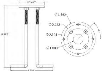
3. Pour concrete and ensure mounting base is flush with concrete.
