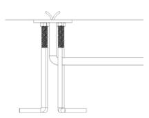
5. Once dry, make electrical connections and attach the mounting plate to the mounting base using 4 M5 screws followed by the base cover plate and fixture.
