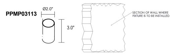
Drill pilot hole for core drilled housing through wall
