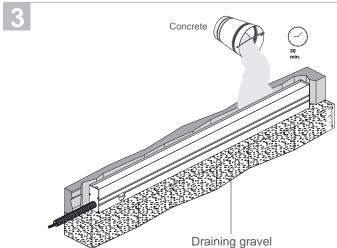
Use 7-12" of drainage gravel - check functionality: fill tube with water and verify full drainage within 30 min. If water remains, please utilize a different drainage system that functions properly. Contractor to seal the conduit with "Great Stuff" aerosol seal that prevents water and moisture penetration for ultimate protection.
