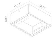
**Standard** (included) Installation system for ceiling 0.35" - 0.47" - 0.59"
