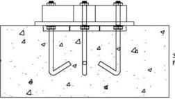
3 INSERT THE PLASTIC BASE AND FIX IT USING 3 NUTS
