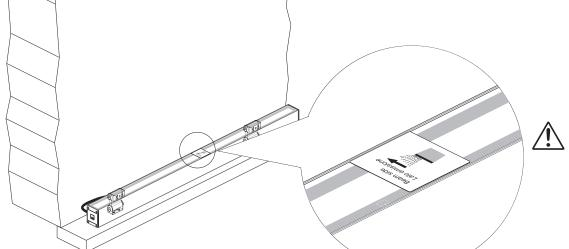
To position the product correctly, use the red label (to be removed after installation) as a reference.
