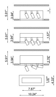
Taurus is an indoor recessed downlight made of Coral® that is available with a single, double or triple rearward spotlight that is extractable and adjustable on both axes. It comes in 3000K as standard with a 22° optic - installable on plasterboard ceilings or walls.
