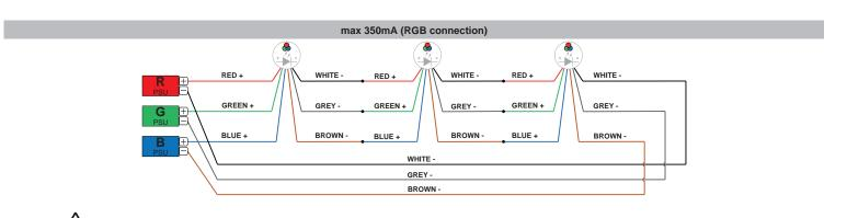
The individual lamps must be connected in series. Only power up the system once all the lamps have being connected.
