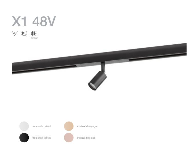
X1 48V is a 48V track light fitting for interiors, available in a black, white, champagne or rose gold anodized finish with interchangeable lenses. Featuring a high-performance projector with a minimal design to have a minimum visual impact, it is fitted with a directional arm 360° adjustable on a vertical axis and 90° on a horizontal one.
