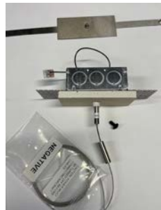
Negative Terminal Leads with Support Boxes
