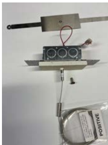
Positive Terminal Leads with Support Boxes
