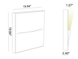
Ready for installation in solid walls Optional plasterkit for installation into **outer casing**
