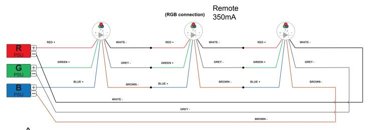
FOR RGB VERSION ONLY: The individual lamps must be connected in series. CURRENT Only power up the system once all the lamps have being connected.
