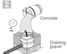
Always Use 7-12" of drainage gravel - check functionality: fill tube with water and verify full drainage within 30 min. If water remains, please utilize a different drainage system that functions properly. Contractor to seal the conduit with "Great Stuff" aerosol seal.
