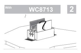
It is the contractor's responsibility to install Remote Driver in a suitable electrical enclosure.
