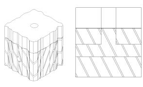
Apply epoxy to sides of newly drilled opening, insert core drilled housing into pilot hole and make level
