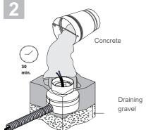
Always Use 7-12" of drainage gravel - check functionality: fill tube with water and verify full drainage within 30 min. If water remains, please utilize a different drainage system that functions properly. Contractor to seal the conduit with "Great Stuff" aerosol seal that prevents water and moisture penetration for ultimate protection.
