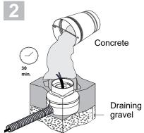
Always Use 7-12" of drainage gravel - check functionality: fill tube with water and verify full drainage within 30 min. If water remains, please utilize a different drainage system that functions properly. Contractor to seal the conduit with "Great Stuff" aerosol seal.
